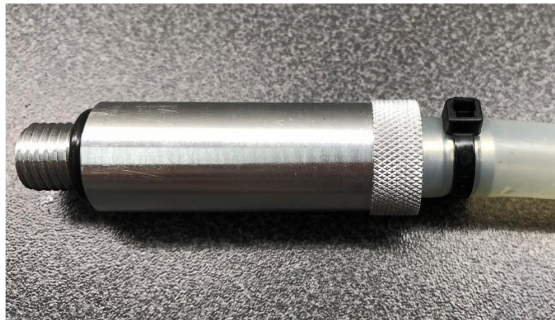
Fig. 1- Zip tie used to secure silicone hose to ODT body
