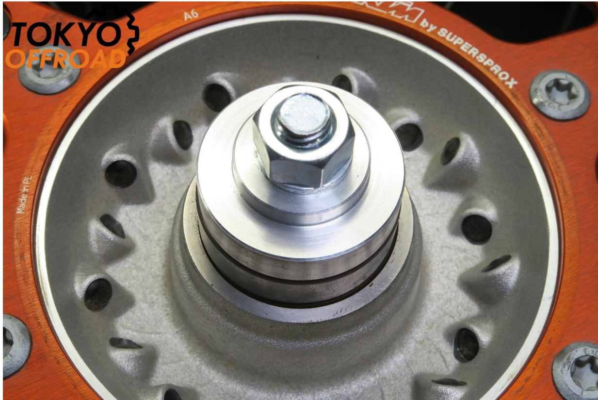
Fig.2- Wheel Bearing Press Tool installed and ready to press in new bearing
