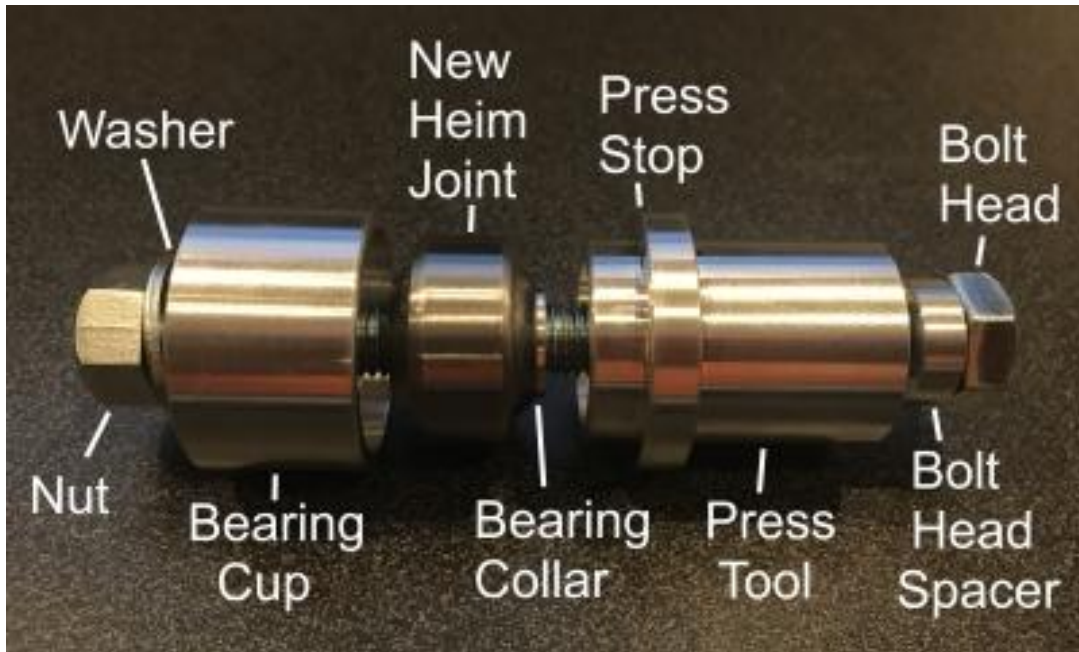
Fig.4- Heim Joint Press Tool installed and ready to press in new bearing
